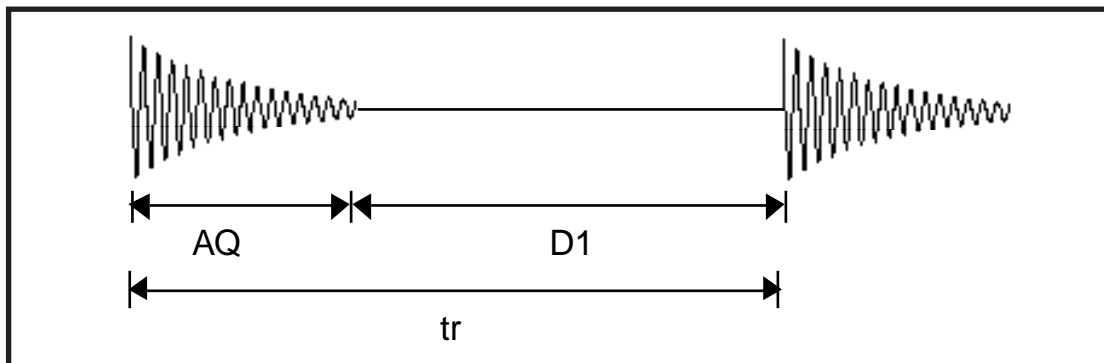
FIGURE 14. Definition of the recycle delay.
